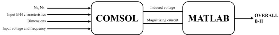
**Figure 2.** The input and output parameters analyzed with the COMSOL Multiphysics and MATLAB.
