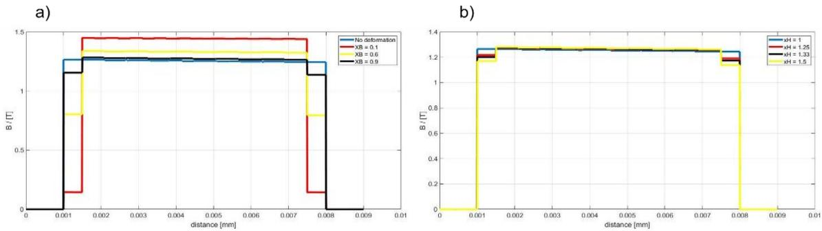
**Figure 8.** Magnetic flux density along the cut line over the ring-core for the variations of: **a)**  $X_B$  and **b)**  $X_H$ .
