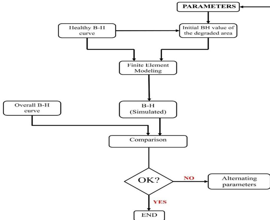
**Figure 4.** The flowchart describes the steps of the proposed algorithm to find the B-H curve of the degraded area.
