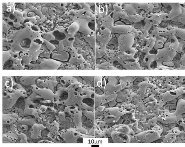
**Figure.3.** SEM images of MAO coated a) 4.7m/min, b) 10 m/min of AZ31-0,2Nd and c) 4,7 m/min and d) 10 m/min of AZ31-0,5Nd.
