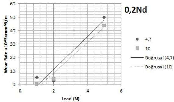
**Figure. 4.** Wear test result of 0,2 Nd added alloys.
