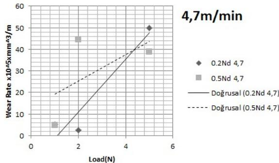
**Figure. 6.** Wear test result of alloys deformed at 4,7m/min rolling speed.
