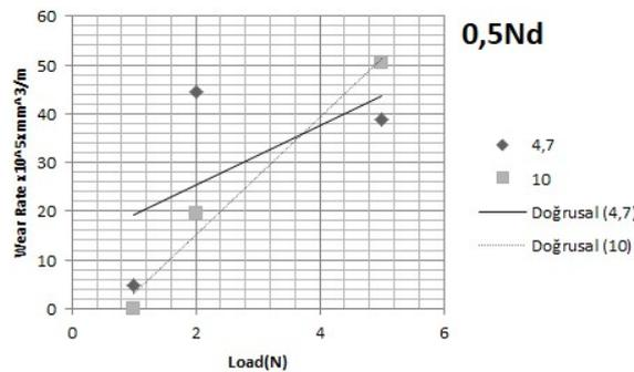
**Figure. 5.** Wear test result of 0,5 Nd added alloys
