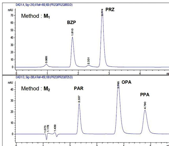
**Figure 1.** Typical chromatograms obtained from standard solutions of OPA, PPA and PRZ (Sample concentrations: PRZ = 3 µg/mL; BZP = 2 µg/mL; PPA = 5 µg/mL; OPA = 10 µg/mL; PAR = 15 µg/mL).
