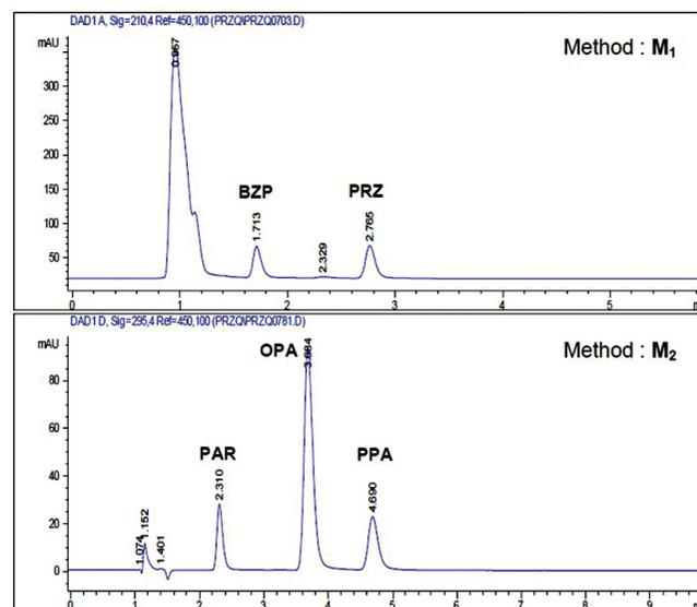
**Figure 3.** Typical chromatograms obtained from the analysis of tablet formulation comprises of OPA, PPA and PRZ.
