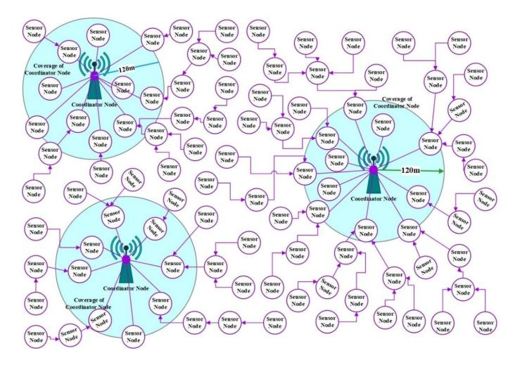
Figure 1. Connection state of Multi-hop Wireless Sensor Networks
