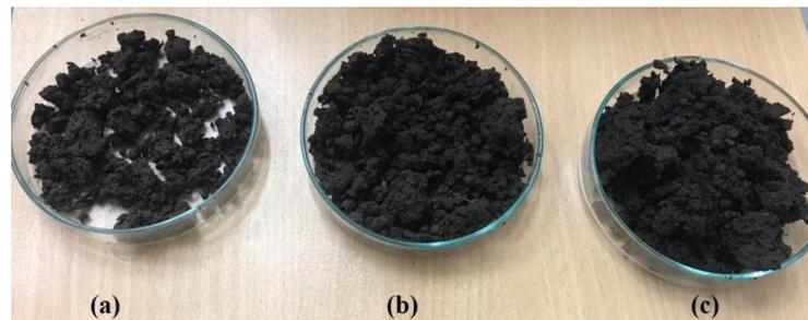
**Figure 3.** Wet sewage sludge samples (a) 20 g, (b) 40 g and (c) 60 g.
