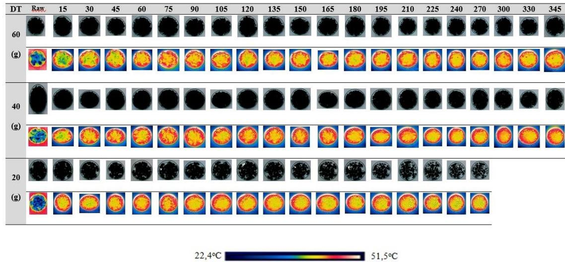
**Figure 11.** Thermal images of raw and dried sewage sludge below 60 °C in conveyor belt drying system.
