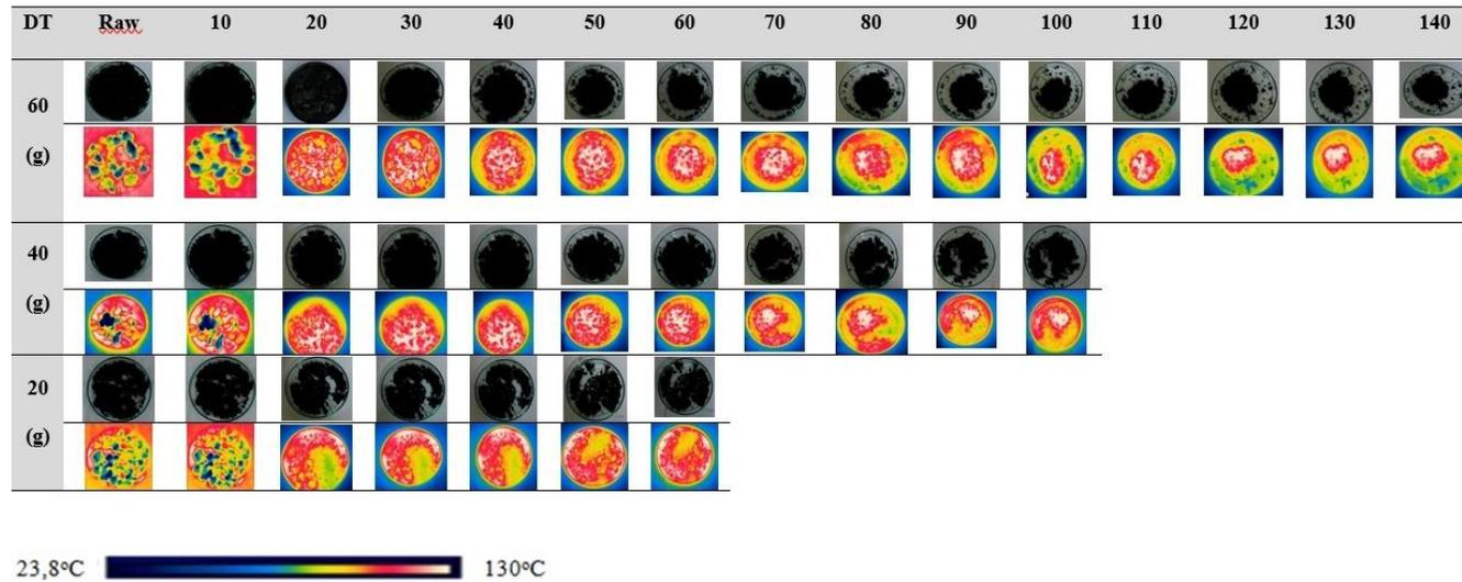
**Figure 8.** Thermal images of raw and dried treatment sludge under 360 W in microwave drying system (DT: Drying Time, minute.).
