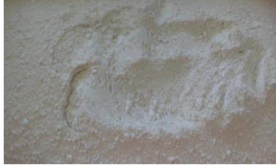
**Figure 1.** Marble powder used in the production of SCLWC samples
