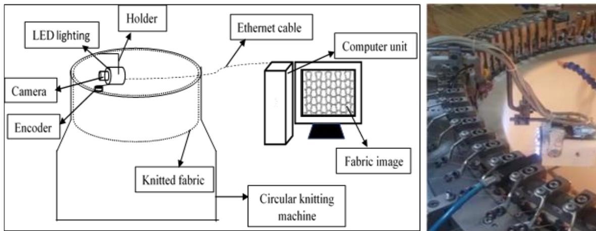
Figure 2. Machine vision system-The circular knitting machine
