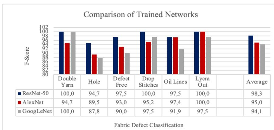
Figure 10. Comparison of the CNNs architectures
