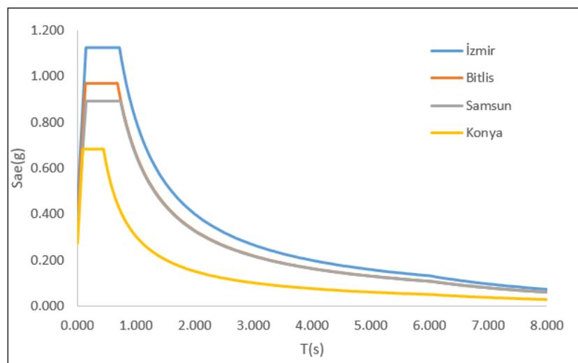
Figure 5. The comparison of horizontal design spectrum
