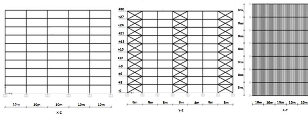
Figure 9. Sections of the sample steel structure model
