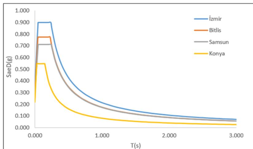
Figure 6. Comparison of vertical elastic design spectra
