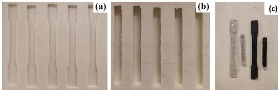
*Figure 1. Mold for (a) flexural bending test samples, (b) Izod impact test samples, and (c) images of produced samples.*
