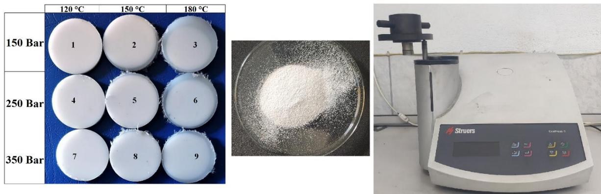
**Figure 1.** Macrostructure photographs of the produced samples, UHMWPE powder, and hot molding device used in experiments
