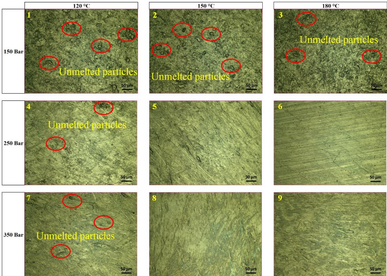
**Figure 2.** Optical microstructure image of the produced samples
