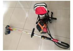
Figure 2. Brushcutter mounted log debarker (B-Debarker)
