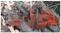
Figure 1. Chainsaw mounted log debarker (C-Debarker)
