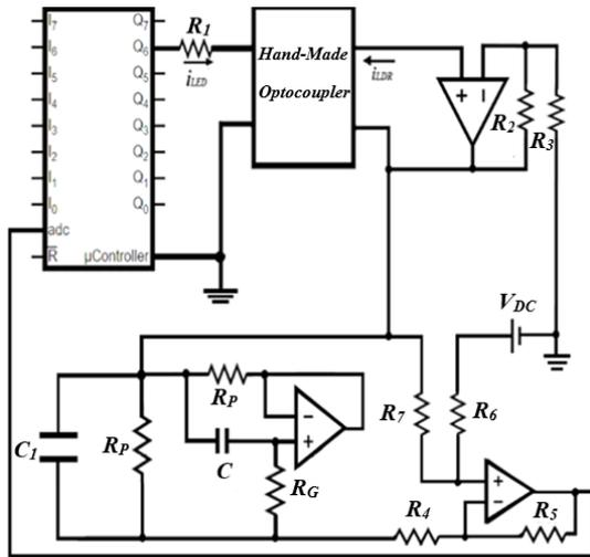
Fig. 8. The Biryukov oscillator circuit schematic
