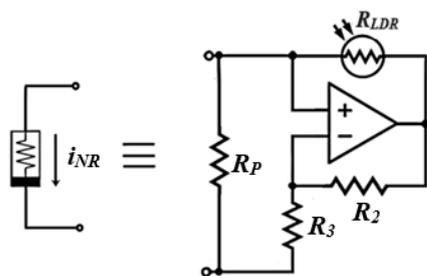
Fig. 6. The nonlinear resistor of the Biryukov oscillator
