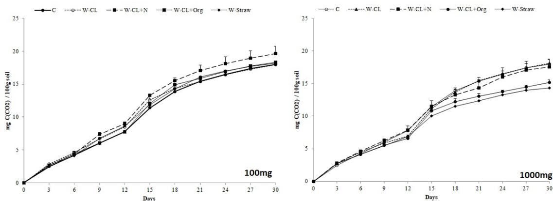
Figure 2. The carbon mineralization of soils with added W-CL and W-Straw.
