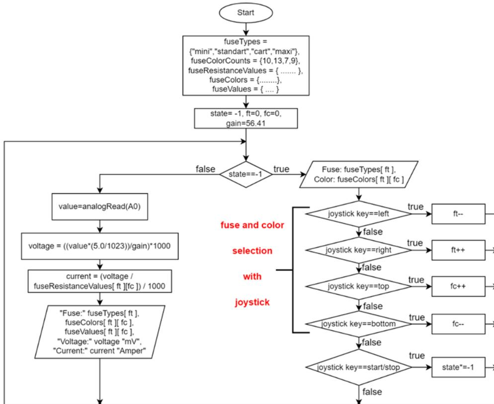
Figure 5. Flowchart of the Fuse Measurement System program.
