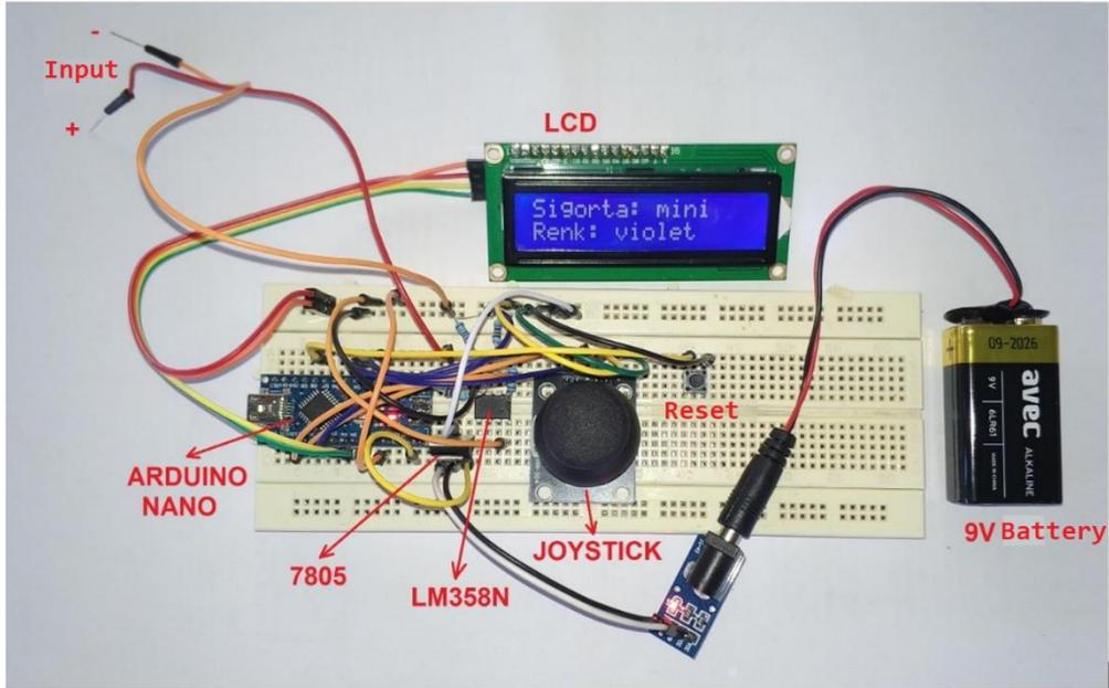
**Figure 3.** The current detection circuit.
