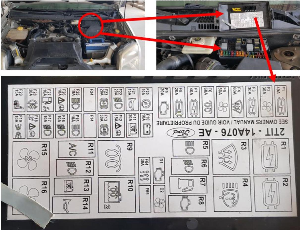
Figure 1. The fuse box under the hood of the vehicle where the experiments were carried out and its cover.
