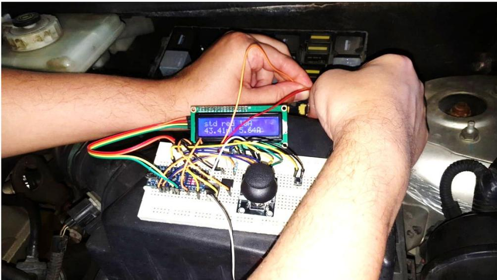
**Figure 4.** The voltage drop measurement with the designed circuit.
