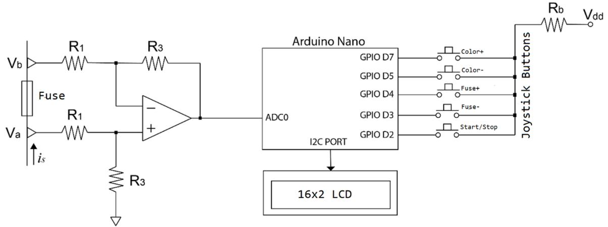
**Figure 2.** The fuse current tester circuit.
