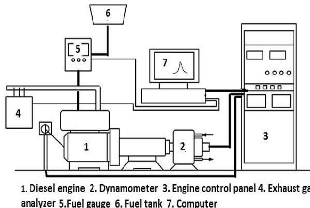
Fig. 1. Test engine is depicted schematically
