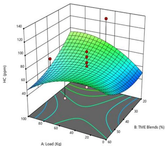
Fig. 8(b). Contour 3D Surface plot with EGR and TME Blends – HC Emission
