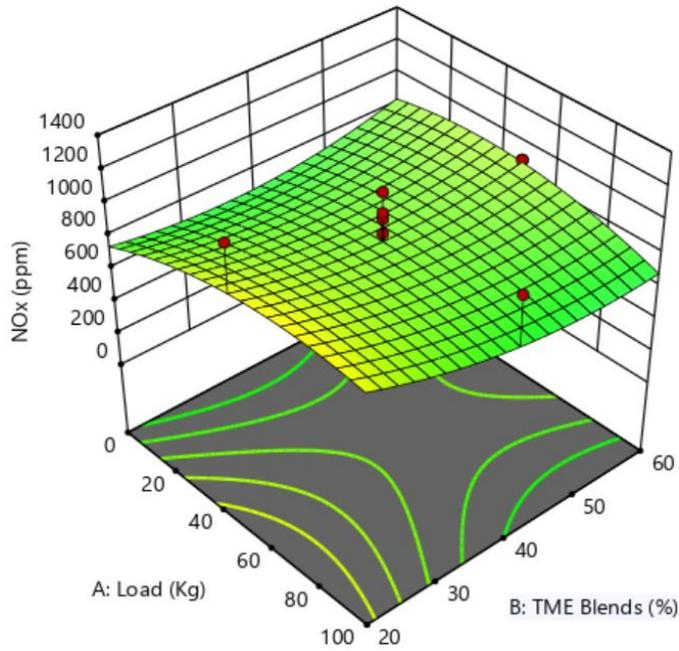
Fig. 10(b). Contour 3D Surface plot with EGR and TME Blends – NoX Emission
