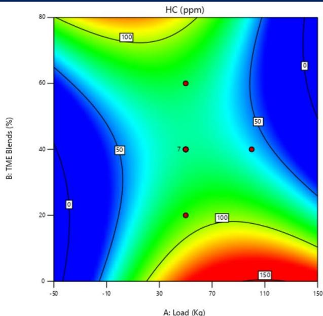
Fig. 8(a). Contour 2D Surface plot with EGR and TME Blends – HC Emission
