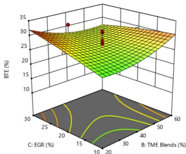
Fig. 2(b). Contour 3D Surface plot with EGR and TME Blends – BTE performance
