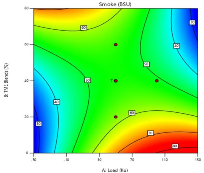
Fig. 12(a). Contour 2D Surface plot with EGR and TME Blends – Smoke Emission
