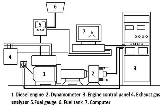
Fig. 1. Test engine is depicted schematically
