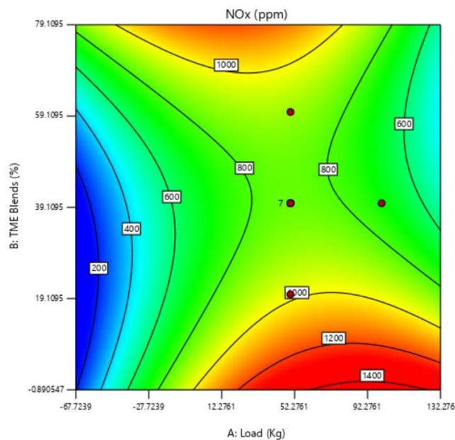
Fig. 10(a). Contour 2D Surface plot with EGR and TME Blends – NoX Emission
