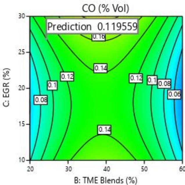
Fig. 6(a). Contour 2D Surface plot with EGR and TME Blends – CO Emission
