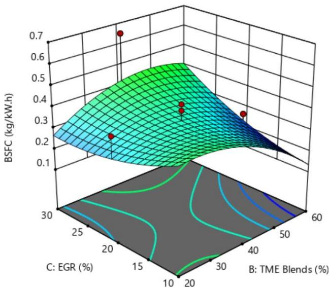
Fig. 4(b). Contour 3D Surface plot with EGR and TME Blends – BSFC performance
