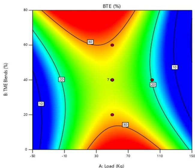
Fig. 2(a). Contour 2D Surface plot with EGR and TME Blends – BTE performance
