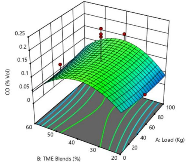
Fig. 6(b). Contour 3D Surface plot with EGR and TME Blends – CO Emission
