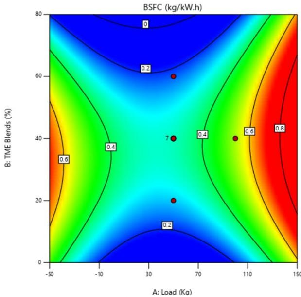
Fig. 4(a). Contour 2D Surface plot with EGR and TME Blends – BSFC performance
