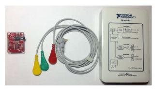
Figure 3. AD8232 ECG module and NI myDAQ card
