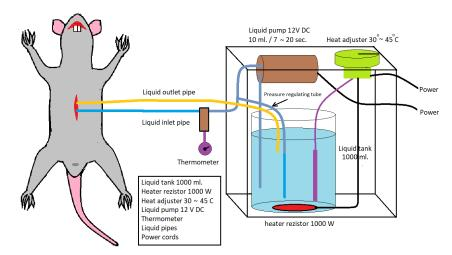
Figure 2. Intraperitoneal infusion pump system working diagram.
