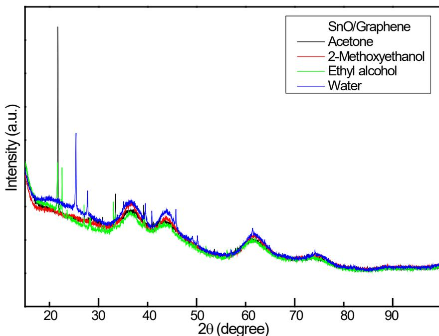
**Figure 2** XRD patterns of SnO/GO nanopowders
