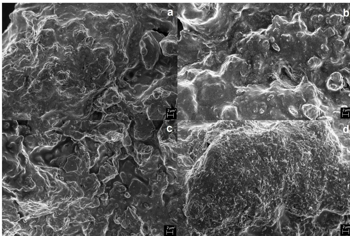
**Figure 1** The SEM images of the a) Acetone, b) 2-Methoxyethanol, c) Ethylalcohol and d) Pure water Hybrid Supercapacitive GO/Sn Nanocomposites
