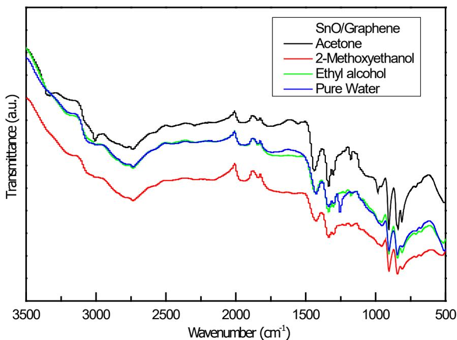
**Figure 3** The transmittance spectra vs. wavenumber of the a) Acetone, b) 2-Methoxyethanol, c) Ethylalcohol and d) Pure water Hybrid Supercapacitive GO/Sn Nanocomposites
