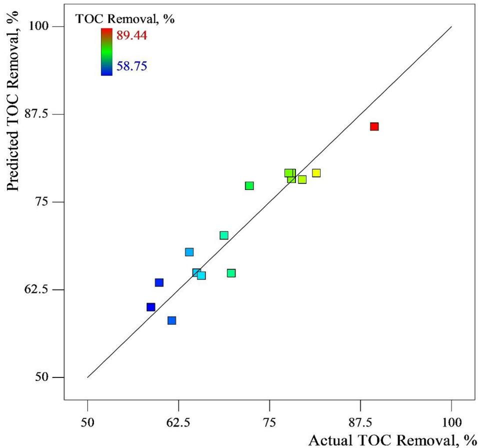
**Figure 1.** Graph of the predicted response values versus the actual response values of TOC removal of MBG.
