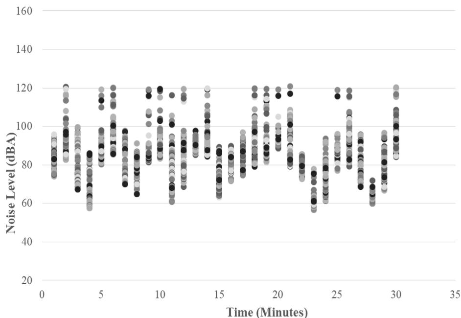
Figure 3. Noise level data measured during skidding operation
