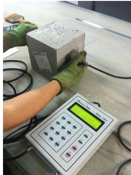
**Fig. 2.** Ultrasonic pulse velocity testing of cubic concrete specimens.
