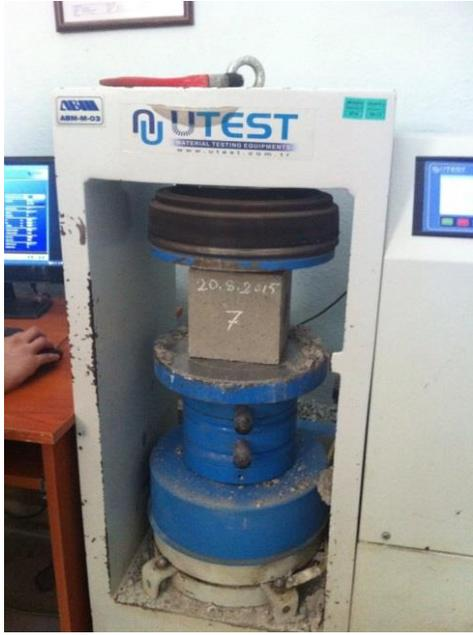
**Fig. 4.** The cubic concrete specimen in the testing machine.
