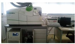
Figure 3. Nexion 300D model ICP-MS
