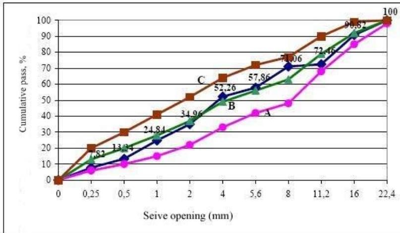
Figure 1. Aggregate granulometric boundary curves depending on the maximum grain
