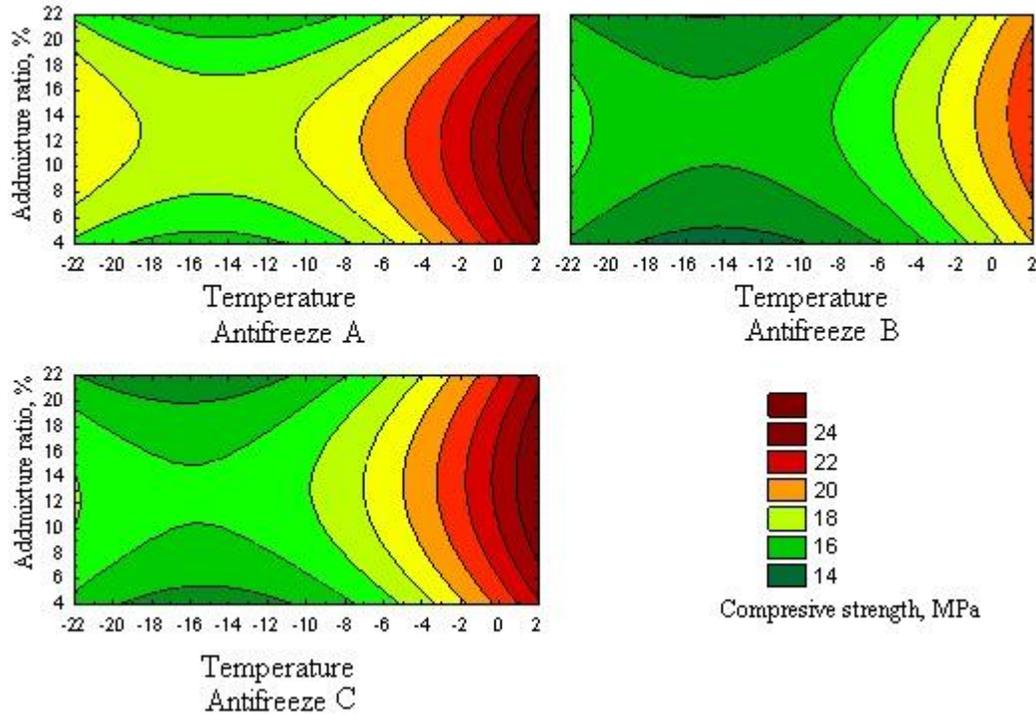
Figure 2. The value of compressive strength of additive A, B and C in concrete samples
