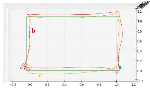
**Figure 5.** Experiment # 5 - 2 (two) drones are drawing a 1m x 1m square at 1m altitude with fixed heading (a-green; given path, b-red and c-orange; measured data)
