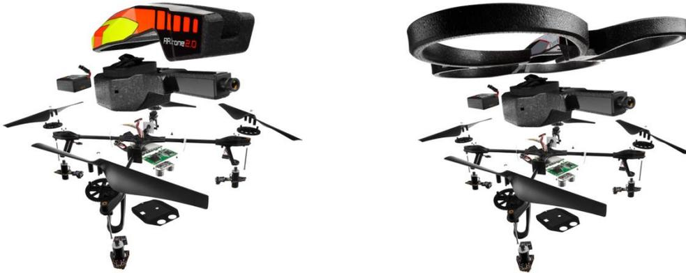
**Figure 1.** AR Drone quadcopter disassembled view
