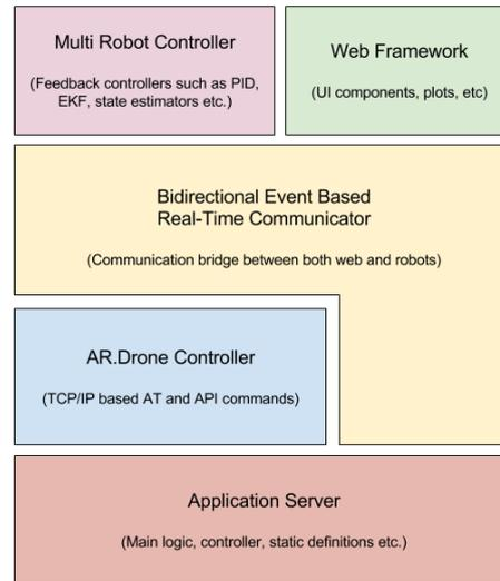
**Figure 2.** “PhDrone” Software Architecture
