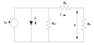
Fig. 5. The simplified equivalent circuit of PV
