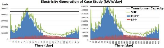
Fig. 9. The electricity generation of the irregular flow based SHE system (1st scenario)
