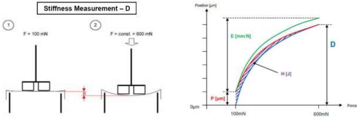
**Figure 4.** Measurement of the stiffness, elasticity, hysteresis and plasticity values [33]
