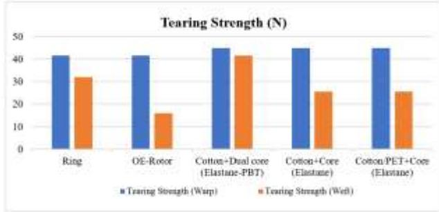
**Figure 9.** Tearing strength of denim fabrics
