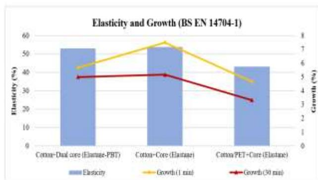
Figure 12. Elasticity (%) and growth (%) values in weft direction of denim fabrics (BS EN 14704-1)
