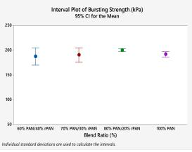
Figure 7. Bursting strength results of yarn samples
