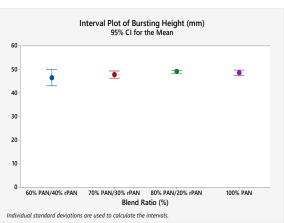
Figure 8. Bursting height results of yarn samples
