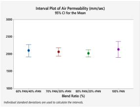
Figure 6. Air permeability results of yarn samples
