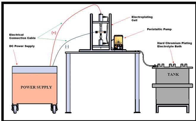
Figure 1. Electrolytic hard chromium plating setup
