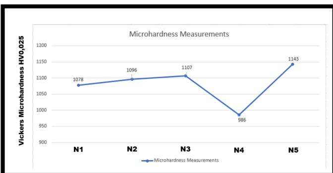
Figure 6. Coating microhardness distribution along the barrel length
