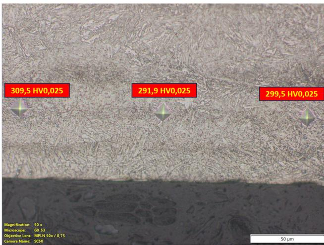
Figure 4. Initial microhardness of low alloy 42CrMo4 steel barrel material
