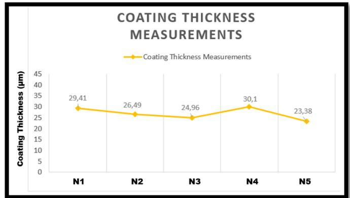
Figure 7. Coating thickness variation along the barrel length
