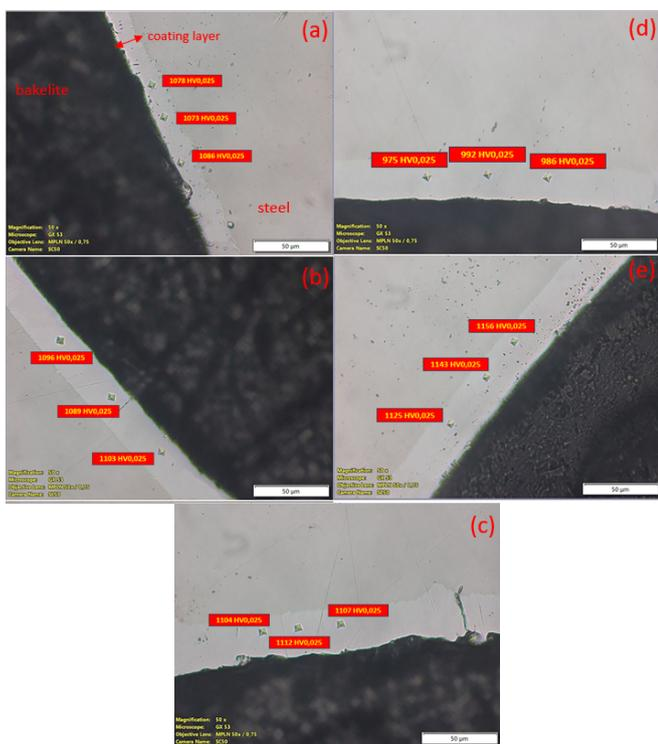
Figure 5. Microhardness measurements along the barrel length; (a) N1, (b) N2, (c) N3, (d) N4, (e) N5 sample
