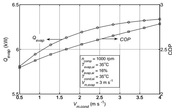
**Figure 10.** The ANFIS predictions for the cooling capacity and coefficient of performance as a function of the mean air velocity at the condenser outlet.
