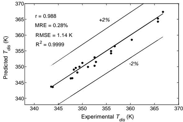
**Figure 7.** The ANFIS predictions for the compressor discharge temperature vs. experimental values.
