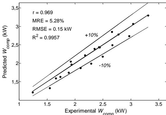
**Figure 4.** The ANFIS predictions for the compressor power vs. experimental values.
