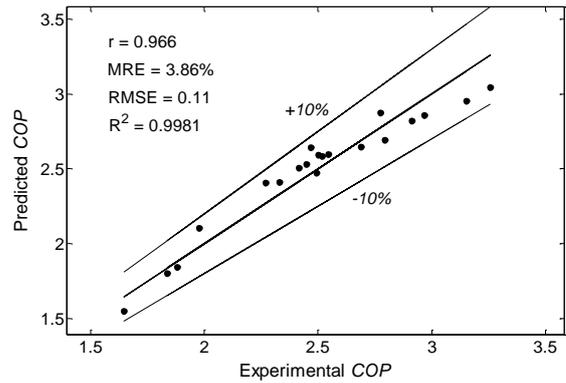
**Figure 5.** The ANFIS predictions for the coefficient of performance vs. experimental values.
