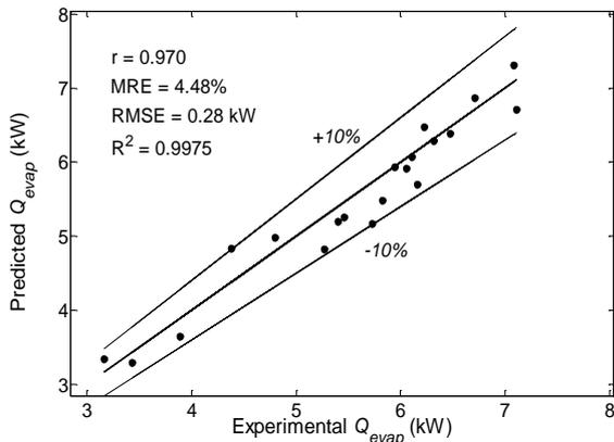
**Figure 3.** The ANFIS predictions for the cooling capacity vs. experimental values.
