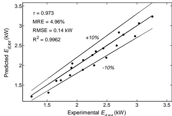
**Figure 6.** The ANFIS predictions for the total rate of exergy destruction in the refrigeration circuit of the refrigeration system vs. experimental values.
