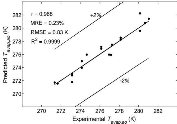
**Figure 2.** The ANFIS predictions for the air dry bulb temperature at the evaporator outlet vs. experimental values.
