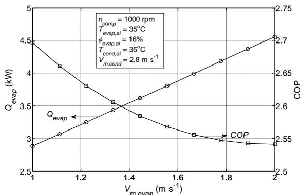
**Figure 9.** The ANFIS predictions for the cooling capacity and coefficient of performance as a function of the mean air velocity at the evaporator outlet.
