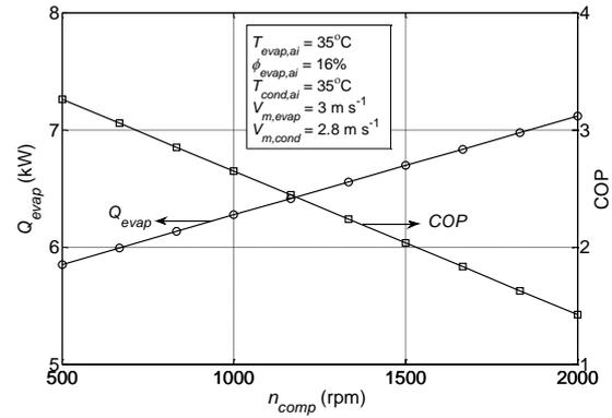
**Figure 8.** The ANFIS predictions for the cooling capacity and coefficient of performance as a function of compressor speed.
