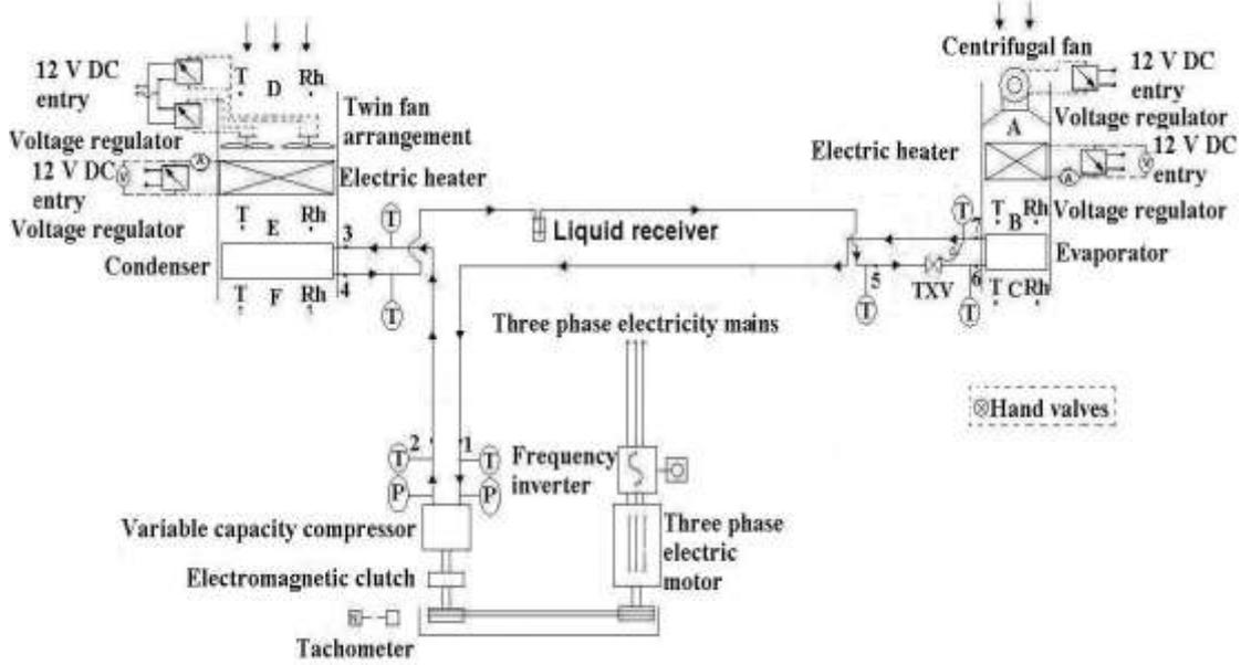
**Figure 1.** Schematic diagram of the experimental AAC system.
